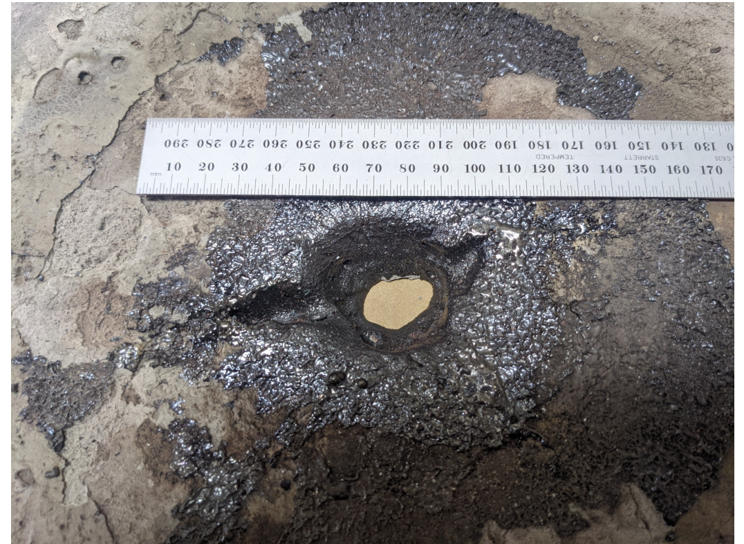
Single Lunar Paver (SL1) Re-Re-Fired
