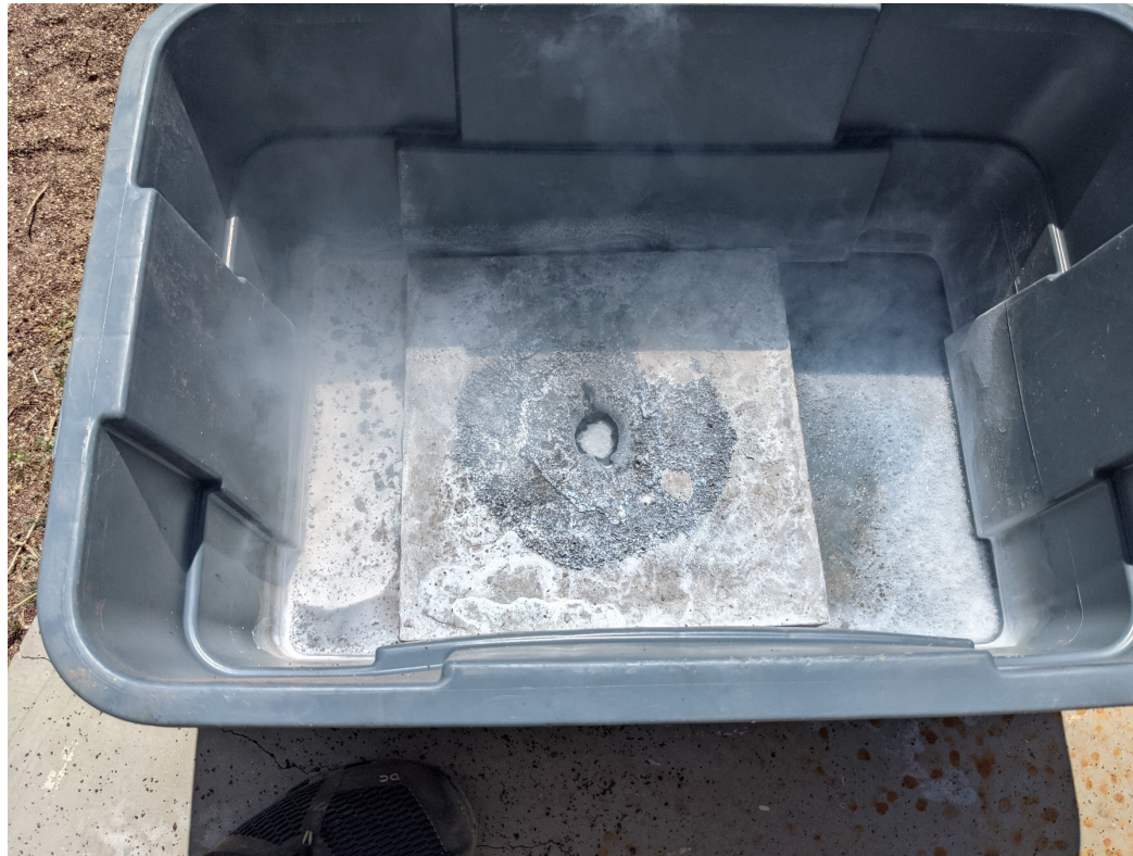
Single Lunar Paver (SL1) 10-min LN2 Soak
